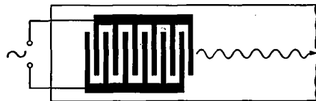
Fig. 1. Interdigital electrodes on a slice of a piezoelectric material (interdigital transducer) for the generation of elastic surface waves. The temporal frequency of the applied a.c. voltage, and the spatial frequency of the 'fingers' must correspond to the frequency and the wave number of the wave to be excited.
