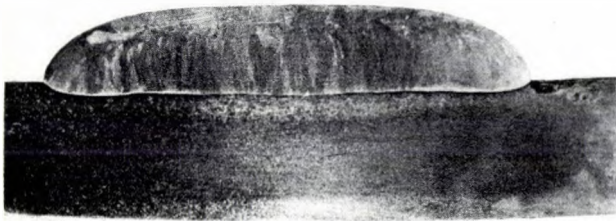
Fig. 6. Weld bead of stainless steel (filler wire PZ 6061, diameter 1.2 mm) on a 10 mm steel plate. Plasma gas 6.5 l argon per minute, shielding gas 12 l argon + 3 l CO 2 per minute. Nozzle diameter 10 mm, distance from torch to workpiece 22 mm. Plasma-arc current 100 A at 45 V. Current in the filler wire 400 A at 40 V, both electrodes are positive with respect to the workpiece. Travel rate 23 cm/min, deposition rate 300 g/min, bead width 40 mm.
