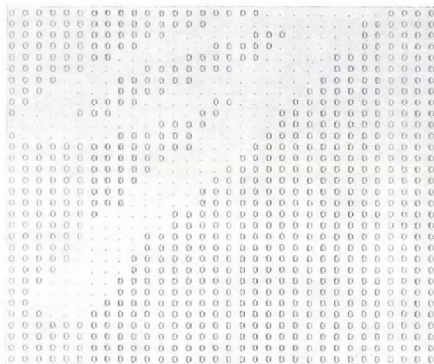
Fig. 13. Matrix with occupied positions (marked with a dot) and unoccupied positions (marked with a zero); the occupied positions represent the numeral nine . In this form the numerals are ready for skeletonization.
